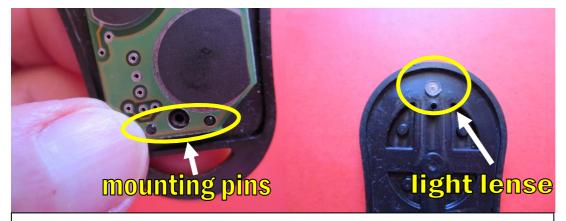
Gently lift up electronic board from 3 mounting pins. When removing electronic board take care not to misplace small clear light lense. Next use flat screw driver to lift light lense from hard shell or a finger nail.
