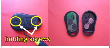
Unscrew 2 small screws at the back of plastic shell. Open remote and separate in 2 parts first: top hard shell part with button key pad and electronic board and second part of hard shell with two batteries.
