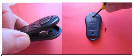
If all components are correctly positioned you can close remote by screwing hard shell together.
