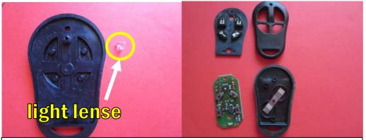
Once lense is removed remove you can push old key pad out from plastic shell using your thumb.
