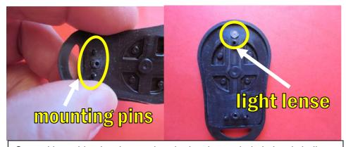
Start with pushing key button thru the key button hole in hard shell and place bottom holes onto respective mounting pins.
