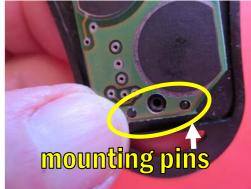
Next place part with mounted electronic board over bottom part of shell. Again holes in electronic board have to be mounted have to go onto mounting pins.
